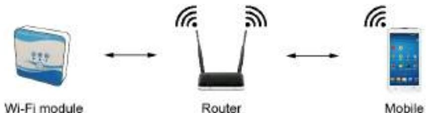
Power on the heat pump unit, the indicators of power and communication on Wi-Fi module will be lighted. Press the configuration button for 3 seconds. When the Wi-Fi indicator keeps flashing, please click the 'Confirm indicator rapidly blink'.
